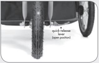
Close the front caliper brake by lowering the Q/R lever. Spin the front wheel to make sure the brake pads do not rub and are properly aligned to the rim. If brake pad alignment is off, loosen brake pad nut with an adjustable wrench, align brake pad and retighten nut while holding brake pad in place.
